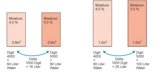
To come to the standard parameter liter per (one) cubic meter, the result with liter per 0.8 cubic meter can be calculated to one cubic meter. I.e.  $64 \text{ Liter} / 0.8 = 80 \text{ Liter/m}^3$ .
